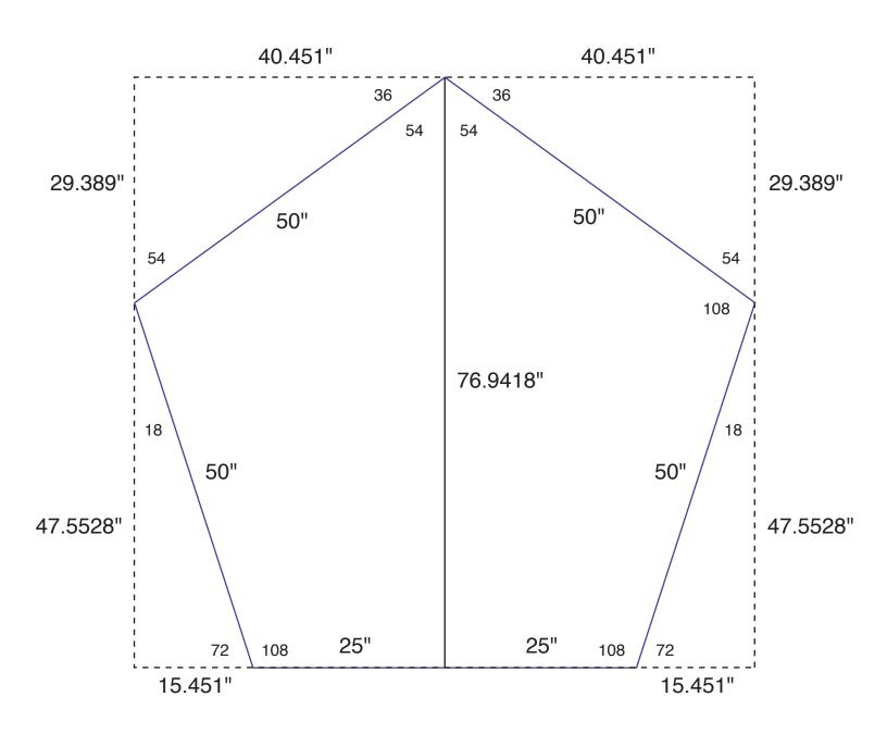
This is the pattern for our interior reflective ceiling. It is made from 2 pentagons taped together around the edges, one of Reflectix insulation and the other tarp. The pentagon is suspended in our dome with the reflective side pointing up. This radiates heat out of our dome, as well as blocks sunlight that pentrates the ventilation screen.
